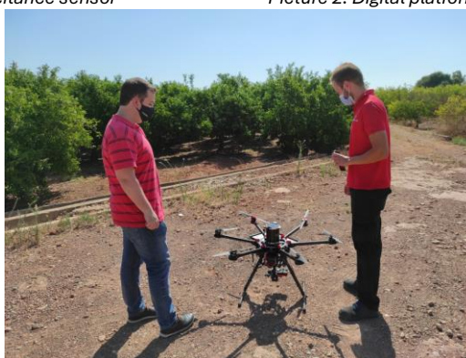
Picture 3. Drone equipped with thermographic cameras
